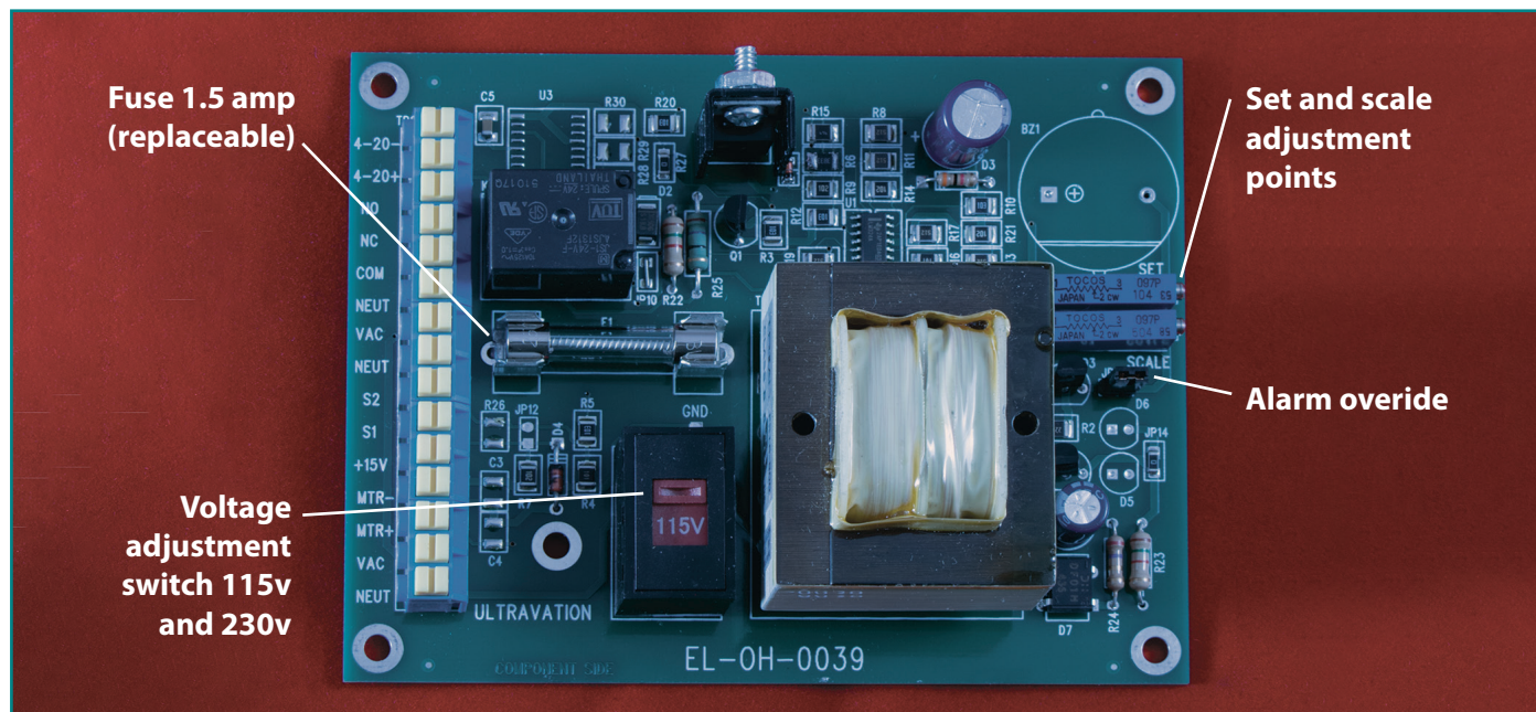
FIG. 2 – UV INTENSITY MONITOR BOARD (ORDER PART NO. 31.0020)
