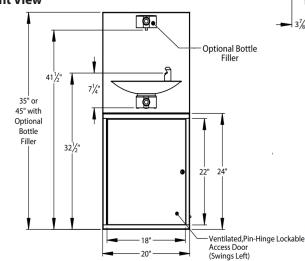
NOTE: Install Chiller in Stud Wall with Minimum 6" x 18" Opening for Exhaust into Plenum Above
