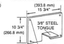
1/4" (6.3 mm) STEEL MOUNTING PLATE
